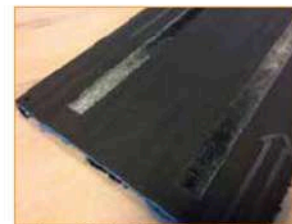
Back tackified adhesive, repositionable.
